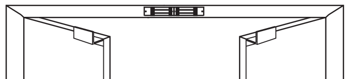
Double Lock, Inswing Door Center Mounted To Header Face With Adjustable Top Jamb "Z" Brackets
