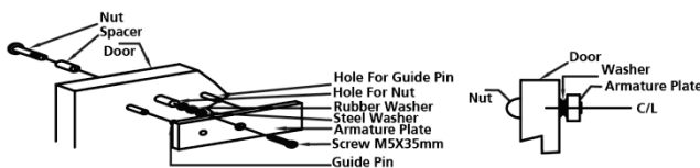
Figure 3: Armature Plate/Surface Mounting
